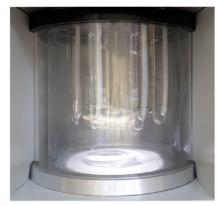
This instrument is suitable for determining the dynamic viscosity of petroleum asphalt by vacuum decompression capillary viscometer method. Unless otherwise specified, the test temperature is 60  $^{\circ}$  C and the vacuum degree is 300mmHg. The vacuum degree and test temperature of the instrument can be set independently, and it is also suitable for other non-standard tests.
