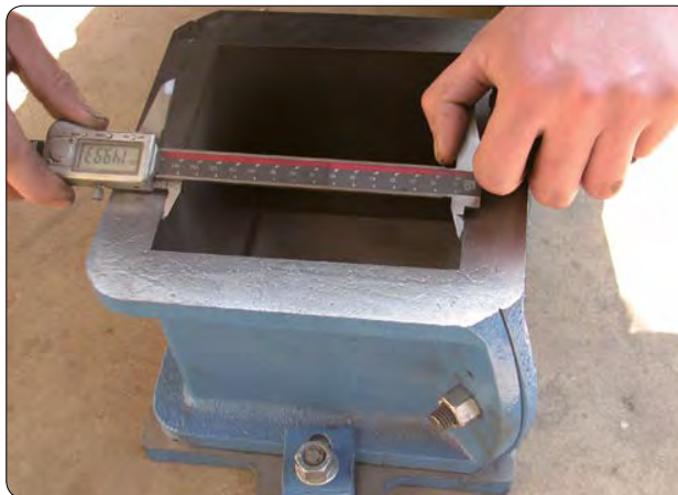
Verification of dimension using digital vernier caliper
