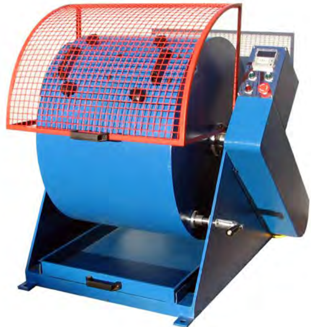
42-5305/01 Los angeles abrasion machine with protect cover
