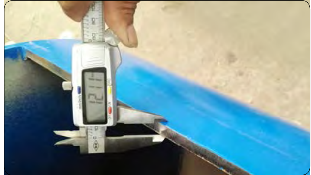
42-5305/01 Los angeles abrasion machine with 12mm wall thickness
