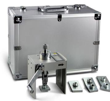
Used to test the bonding strength of decorative bricks, tiles, mosaics, various plates, paints, coatings, exterior wall insulation materials (EPS panels, SPS panels), and also be used to test the bonding strength of various exterior wall building materials and adhesives.
