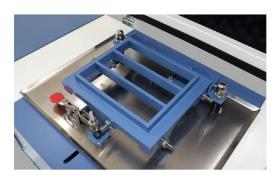
Jolting Table is used for compacting of cement specimens in 40x40x160mm three gang mould. It consists of a table holding the mould, seated on a rotating cam driven at 60 rpm. The jolting group is connected to the table by bayonet joints for quick checking of the weights. The drop height 15.0 mm is adjustable to keep it correct also after intensive uses.
