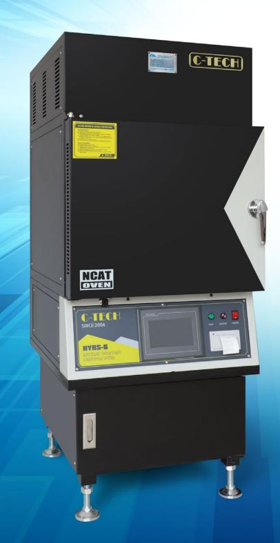
The asphalt content ignition oven HYRS-6 is a micro controller based equipment based on the electric ignition oven method for fast and accurate determination of asphalt content.
