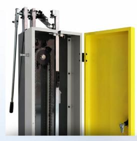
The Marshall compactor EDC-3A is used to make asphalt mixture specimens by standard compaction method for testing the physical and mechanical properties of asphalt mixture in the laboratory. It is suitable for the forming of  $\Phi$  152.4mm ( $\pm 0.2$ mm)  $\times$  115mm /  $\Phi$ 101.6mm ( $\pm 0.2$ mm)  $\times$  63.5mm cylindrical specimens used in Marshall test and indirect tensile test. EDC-3A has a manual lever hammer lifting device and two sizes of hammer weight.
