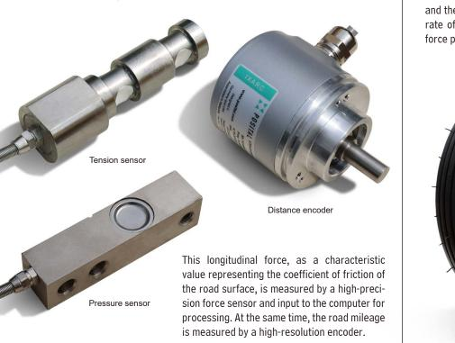
Due to the speed difference between the test wheel and the road wheel, the test wheel generates a slip rate of 12-17%, which will generate a longitudinal force perpendicular to the driving direction.
