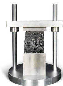
IDEAL RUTTING TEST (IRT) ASTM WK71466 ASTM D8360
