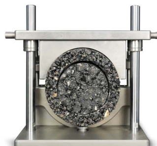
TACK COAT/INTERLAYER BOND STRENGTH TEST (DIRECT SHEAR TEST) EN 12697-48 AASHTO TP114
