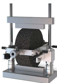
INDIRECT TENSILE TEST EN 12697-24 METHOD F
