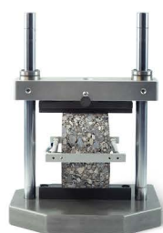
INDIRECT TENSILE TEST EN 12697-24 METHOD E
