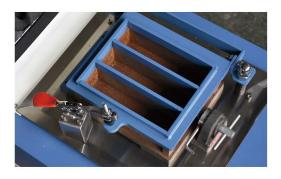
Jolting Table is used for compacting of cement specimens in 40x40x160mm three gang mould. It consists of a table holding the mould, seated on a rotating cam driven at 60 rpm. The jolting group is connected to the table by bayonet joints for quick checking of the weights. The drop height 15.0 mm is adjustable to keep it correct also after intensive uses.
