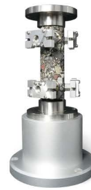
DIRECT TENSION TESTING AASHTO T411
