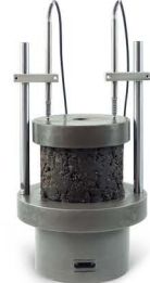
UNIAXIAL COMPRESSION TEST
