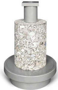
UNIAXIAL PENETRATION TEST
