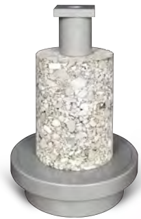
Uniaxial penetration test (D50) kit JTG D50 Appendix F
