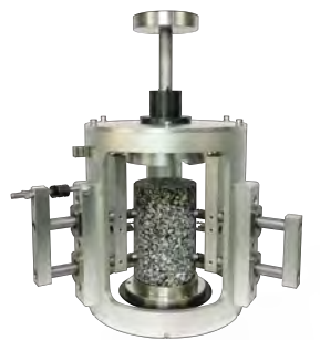
Dynamic modulus test specimen preparation auxiliary device
