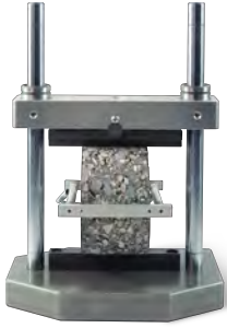
Indirect tensile fatigue test kit EN12697-24 Method E
