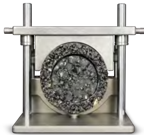
Shear bond test kit EN12697-48
