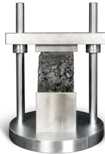
Ideal rutting test (IRT) kit ASTM WK71466, ASTM D8360
