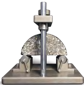
Semi-circular bend (SCB) test kit AASHTO T393, ASTM D8044
