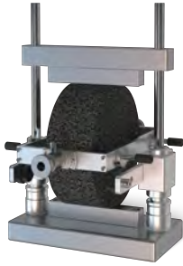
Indirect tensile fatigue test kit EN12697-24 Method F
