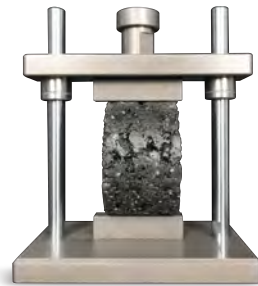
Tensile splitting test kit JTG 3410 T0716
