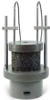
Uniaxial compression test kit JTG E20 T0713
