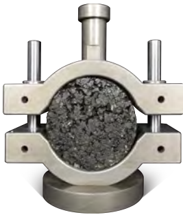
Marshall stability test jig JTG E20 T0709
